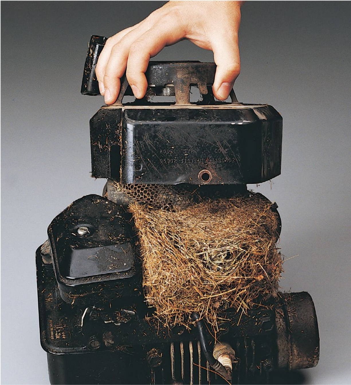
To fully remove all the debris buildup (the photo above shows a fairly advanced case) often means doing some light disassembly to gain full access to the areas where debris collects.
